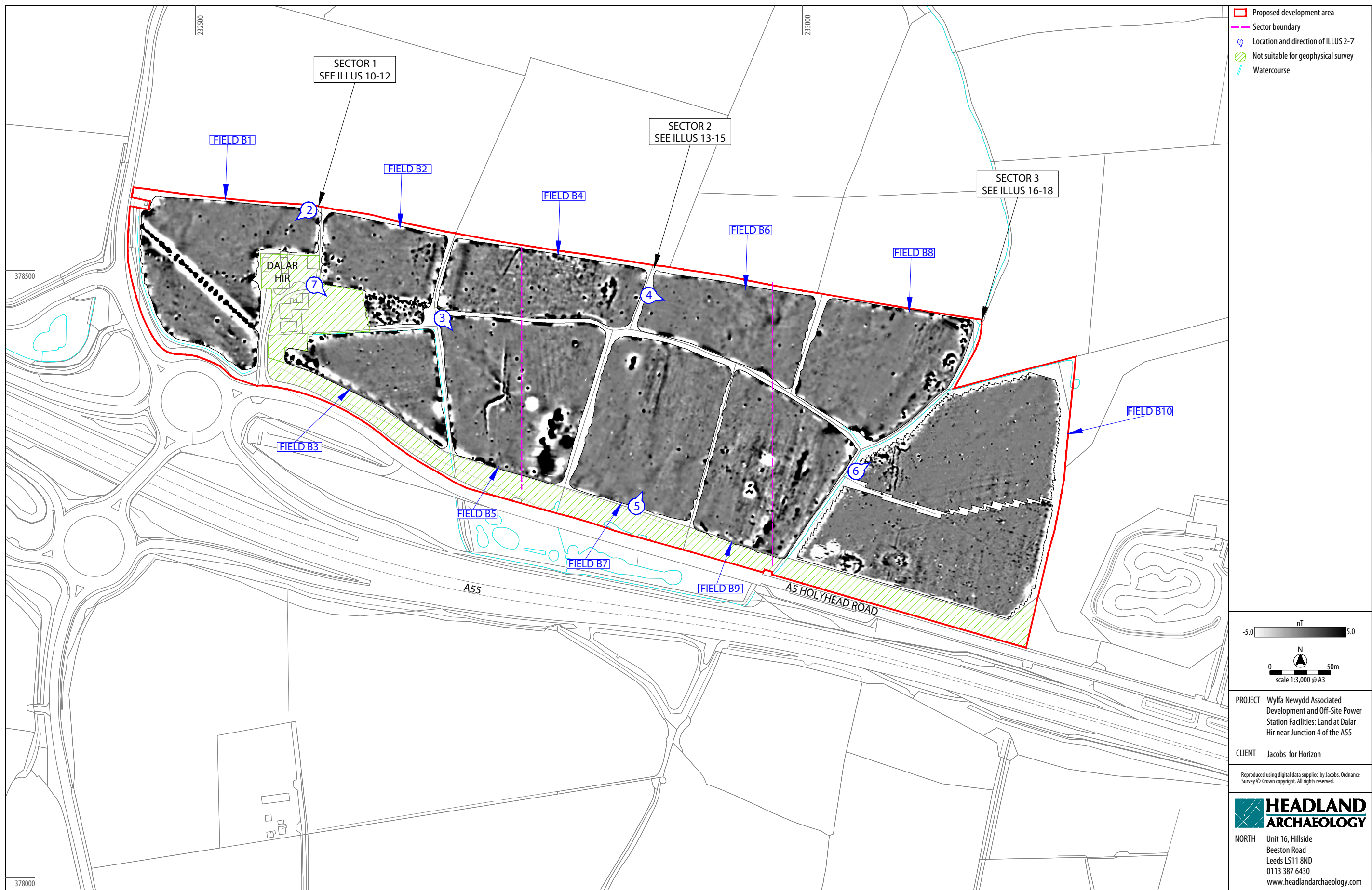
Illus 8 Survey location showing greyscale magnetometer data
